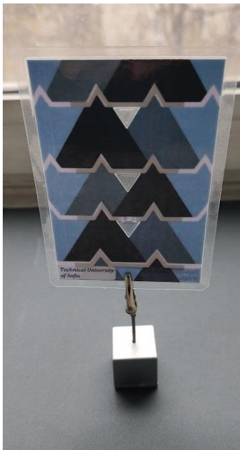
fig. 4 – Prototype of directional WiFi antenna
